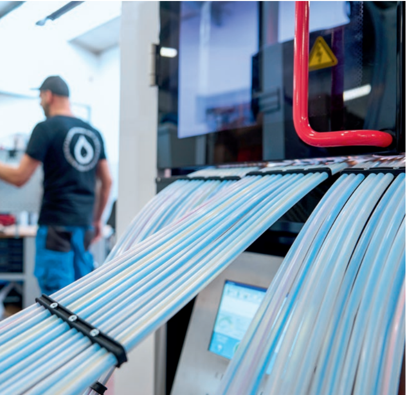
Based on the digital twin, the Wire Terminal produces a complete set of cables for an enclosure in one hour.
