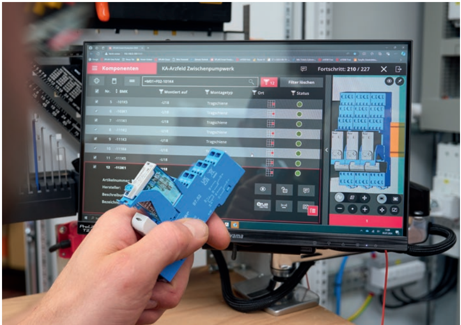
Eplan Pro Panel is used to create the enclosure's digital twin, which then provides the basis for manufacturing with Smart Mounting.
